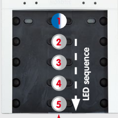
Pattern 1 (MX-Bell1-Button-F1): LED 1 permanently blue (function button) LEDs 2 to 5 flashing white 4 (bell buttons)
