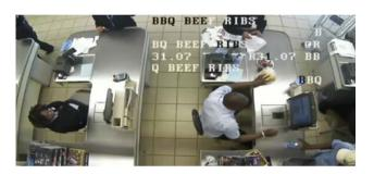
Hikvision's POS Solution connects surveillance video with transaction data at Points of Sale (POS). All scanned items can be displayed in live view and playback and can be programmed to trigger alarms. This allows managers to instantly playback or search for a specific transaction – even months after the event. This resourceful solution serves to reduce hidden shrink from theft or fraudulent POS activity.
