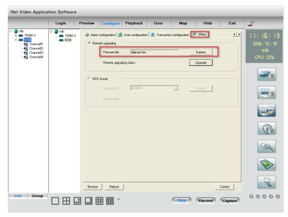
Fig.4.8 Remote upgrading
