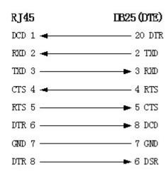
(2) 25-pin to 9-pin converter's internal connection is like this:
