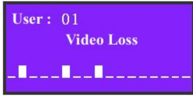
Fig 2.3.13 Video Loss Alarm
