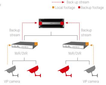
NVR/DVR can back up VIP camera channel recording in real time to Blazer Pro, so there will be 2 video footage of VIP cameras for safer recording.
