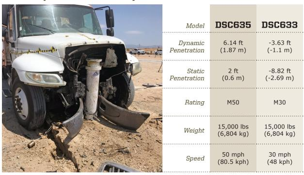
Delta Scientific's new patent pending DSC633 and DSC635 single shallow foundation bollards provide the highest level of protection against a vehicle attack. Tested to the new F2656-20 ASTM M30 and M50 standards, these new bollards provide the stopping power needed for today's threats. With a shallow foundation of only 24 inches (60.96 cm) and the ability to have single units, both bollards offer the flexibility and ease of installation for your perimeter needs.
