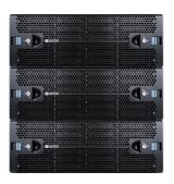
Up to 254 network cameras can be connected to each PetaBlok, which are supplied with pre-installed Wavestore's Video Management Software (VMS). Throughput options up to 2,400Mbits/sec are available, with multiple network interfaces to segregate incoming and outgoing network traffic. Ports can be bonded to provide fault-tolerance and maintain the highest levels of performance at all times
