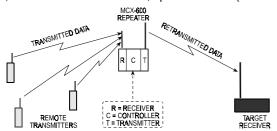
Figure 1. Single-Level Repeater Configuration
