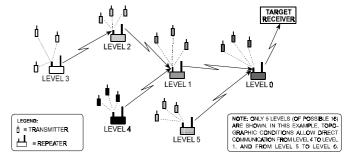
Figure 2. Multi-Level Repeater Configuration
