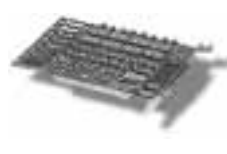
I/O board for alarm handling with 8 opto-isolated inputs and 8 relays output
