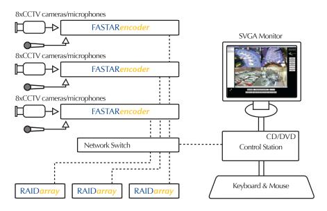
RAIDarrays networked with FASTARencoders to provide a 24 channel system
