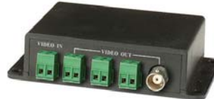
TA1013CTD 1 UTP in 1 coax out and 3 UTP out
