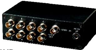
C1008VD 1 in 8 out Coaxial Video Distributor Metal case 133x87x44 mm 450 gm 12Vdc 150 mA
