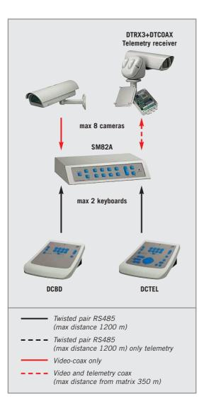
The SM42A-SM82A microprocessor-controlled matrix with remote or local control allows the switching of 4 (8) cameras on 2 video outputs.
