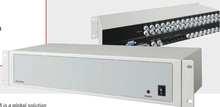
The full cross point video matrix switcher SM328A is a global solution for the collection and management of images. The matrix is capable of switching 32 video inputs to 8 independent outputs. This product can activate 32 different synchronized sequences among several monitors, with day, night or holidays cycles.
