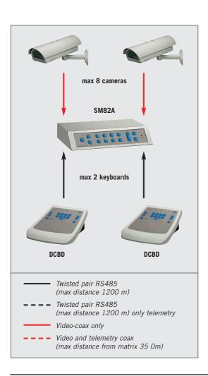
The DCBD keyboard is the solution for remote control of the SM series matrix.
