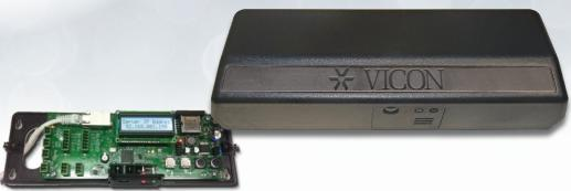
The Vicon Access Control (VAX) system consists of a dedicated Vicon Access Control Server and the edge Controller(s). The Server contains the operating system, database engine, web server, application software and configuration data. The Controller communicates back to the Server over the network and provides an interface to readers, relay outputs, door locks, etc.
