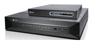
The HDExpress<sup>™</sup> is a plug-and-play Network Video Recorder (NVR) designed specifically for High Definition (HD) IP cameras. The system includes PoE ports, allowing the NVR to provide power directly to each camera, up to a maximum of 16 (model dependant). The software automatically detects and configures the network cameras, eliminating the need to program any settings. A variety of 4, 8 and 16-channel units are available with a choice of storage capacity.
