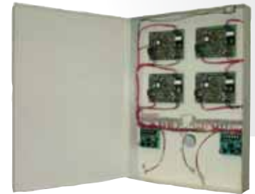
8-door controller (large cabinet)
