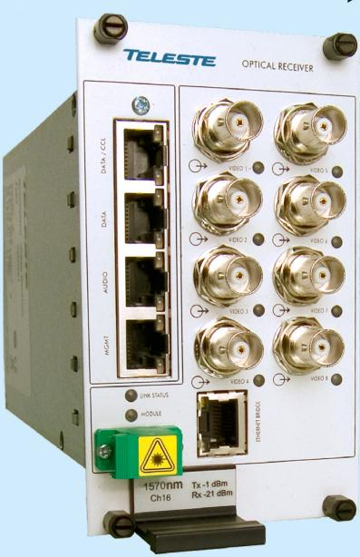
New CEV video modems are basic building blocks for multi-channel video transmission system providing unidirectional transmission of 8 zero-delay video channels together with bi-directional audio, data, contact closure and Fast Ethernet channels over one singlemode fibre.
