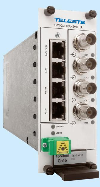
New CEV video modems are basic building blocks for multi-channel video transmission system providing uni-directional transmission of 4 zero-delay video channels together with uni-directional audio, data and contact closure channels over one singlemode fibre.
