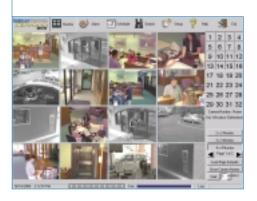
Customized recording. Though XPress DVX is set to record straight out of the box with its default settings, you can easily set your own recording schedule and method. The most efficient recording method is motion (or activity) detection. Specific cameras can be set to record on alarms, enabling complete customization of alarm recording rates and resolution. Maximum recording rate is 60 images/second (50 in PAL).
