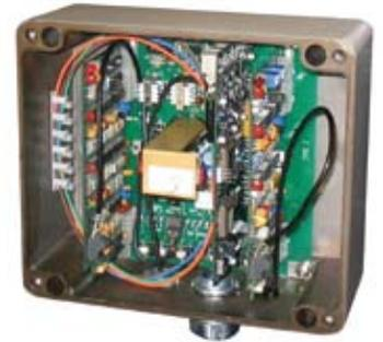
Each FPS-5 processor validates the communication packet before re-transmitting the information to the next processor. The FPS-5 audio signal is digitized and interleaved with the data packets on the same fiber optic cable. This technique eliminates the need for a dedicated audio BUS.
