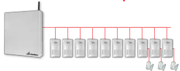
RISCO Bus Wiring
