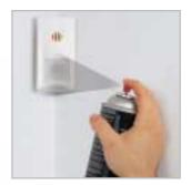
**Masking** is when a would-be intruder physically approaches the detector to cover the **detector's field-of-view** while the alarm system is not armed - in preparation for a burglary.
