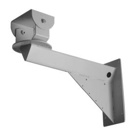
The **WM3026** wall mount has been designed specifically for use with Pelco's heavy duty pan/tilts and/or enclosures. Manufactured from 0.25-inch (6.35 mm) aluminum, the **WM3026** is capable of supporting a maximum load of 300 pounds (136.08 kg) and can be safely mounted to any vertical load-bearing surface.
