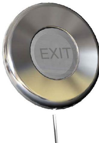
To remove the unit, insert a small screwdriver into the cut out provided and use it to lift the locking pin. The unit can then be rotated anticlockwise to release it from the backplate.
