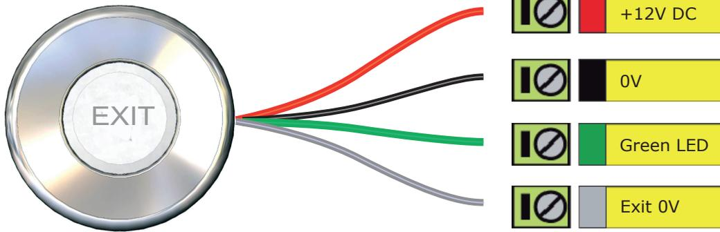
This unit uses solid state electronics to switch 0V to the Exit 0V output and therefore cannot be used with circuits that require voltage free contacts.
