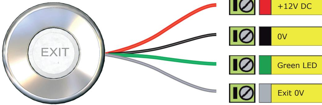
This unit uses solid state electronics to switch 0V to the Exit 0V output and therefore cannot be used with circuits that require voltage free contacts.
