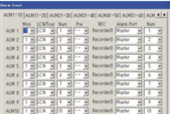
This menu can be used to program which monitor will carry out the spot/tour sequence of a specific camera, when an alarm signal is input.
