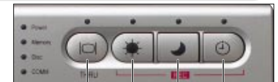
Thru mode button Daytime recording mode button Nighttime recording mode button Timer recording mode button
