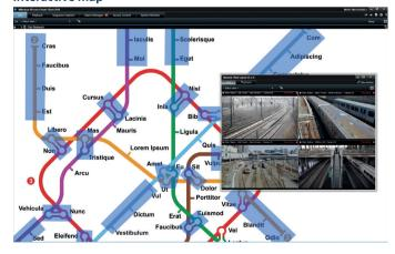
To ensure immediate incident detection, system alarms can notify users of certain events, or if the equipment is malfunctioning. Alarms from all connected security devices and systems are shown in the **interactive map** where alarms from sub-maps are propagated to the primary map.
