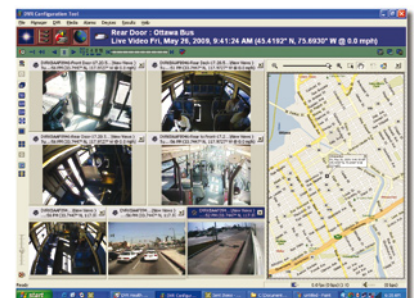
GPS-based mapping displays vehicle location and speed together with synchronized video
