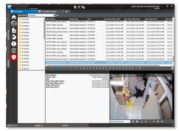
This Security Audit lists all of the alarms that have come in for the various stores, and displays the details and video for the selected alarm (motion detection at the back door)
