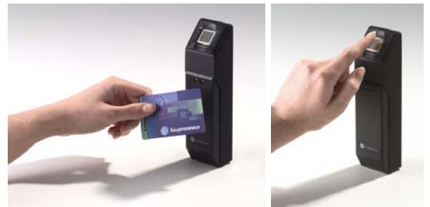
SmartTOUCH™: double verification by card and fingerprint.
