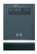
An offline wall reader is the ideal addition to door terminals or electronic cylinders and can be installed for garage doors, roller doors, lifts, motor-powered doors, automatic doors, laboratory equipment, machine controls and other devices. The IP 65 protection class enables use both internally or externally.
