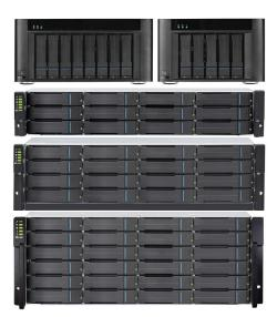
Multiple fans and power supplies in rack mount models provide redundancy to ensure continued usage in the unlikely event of component failure. The RAID controller is hardware-based and controls all logical drive functions transparently to the host system. The storage appliance appears as a standard SCSI drive or drives (in SAN mode) or a network drive (in NAS mode) to the computer's operating system.
