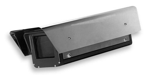
The BPHKIT camera housing has been designed for maximum bullet and tamper resistance. Each housing is constructed of heavy duty extruded aluminum with a 3mm stainless steel armored plate on each side to provide maximum protection from side impact. A 3/4 inch Lexan® window provides maximum protection against front impact. A stainless steel collapsible sunshield further protects the sides and the top of the housing.
