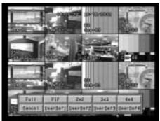
Simply move the mouse to the bottom of the main monitor screen and the various display options are shown. Choose between a full screen view, PIP1, PIP2, PIP3 (Picture in Picture), 2x2, or any of the four customizable user-definable views.
