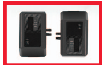
Fiber Optic Link – Network (FLN) Pair
