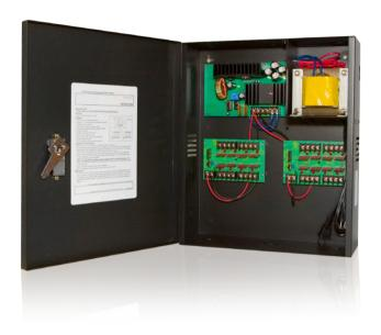
The PWR-12DC-16-10 is a CCTV power center engineered to manage remote camera and accessory power requirements. This distribution module is designed with 16 individually fused outputs for powering up to 16 CCTV cameras and accessories. It will provide 12 VDC via distribution to sixteen fused outputs with a total of 10 Amps continuous supply current. The PWR-12DC-16-10 power center is housed in the premium lockable heavy gauge metal enclosure.
