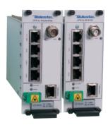
CF0161 series video link consist of a transmitter - receiver pair communicating over one singlemode fibre.
