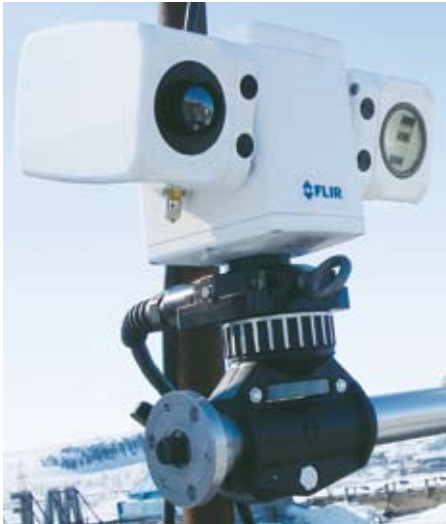
The PTZ-35 MS and PTZ-50 MS can be easily installed in existing CCTV networks.
