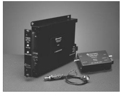
Fiber Options' Series 112V Video System transmits standard video signals. A complete Series 112V System consists of a miniature video transmitter (part number 112V-T) and a modular or rack-mounted receiver (part number 112V-R or 112V-R-R). The transmitter has been designed specifically for easy installation near CCTV cameras enclosed within environmentally secure housings.
