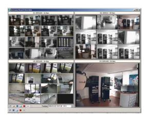
Multiview function enables display of up to 256 cameras from up to 16 different DVRs
