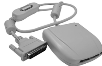
EDA 959 – CompactFlash card adaptor parallel for PC
