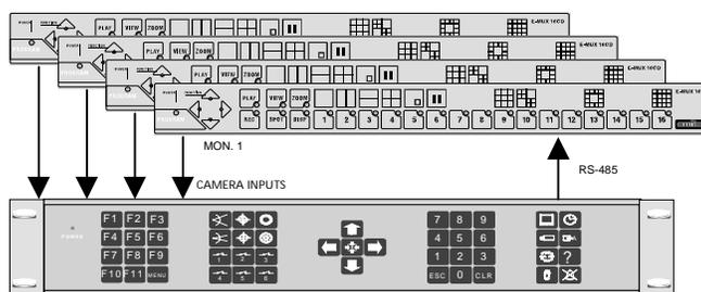
One or more E-MUXs can easily be integrated with the 500M or 1000M video matrixes.
