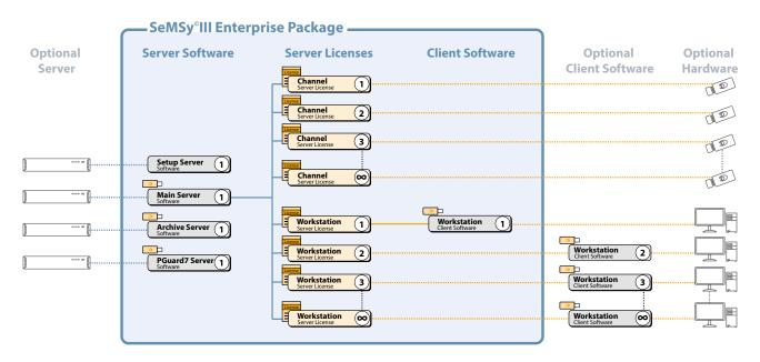
The SeMSy® management system is designed as an open platform for the integration of 3rd party systems. In connection with Dallmeier recording systems 3rd party network cameras compliant with the ONVIF standard can be integrated into the video surveillance installation In addition, the optional SeMSy® III Interface Server Software provides a standardized interface for data exchange with 3rd party POS, access controls or dealing shoes.
