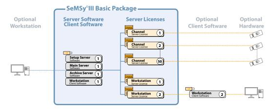
The SeMSy® management system is designed as an open platform for the integration of 3rd party systems. In connection with Dallmeier recording systems 3rd party network cameras compliant with the ONVIF standard can be integrated into the video surveillance installation In addition, the optional SeMSy® III Interface Server Software provides a standardized interface for data exchange with 3rd party POS, access controls or dealing shoes.
