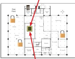
An embedded floor plan graphic allows you to locate CyberLock devices within a specific location. To view a specific device, simply click and zoom in. By viewing the floor plan you can spot 'holes' in access control implementations.
