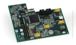
The ComNet™ FVT1031(M,S)1-P series video transmitter along with the ComNet™ FVR1031 series receiver supports simultaneous broadcast-quality video transmission of 10-bit digitally encoded video and return RS422 or Extended Distance Coaxitron data over one multimode or single mode optical fiber. The unit is designed to plug directly into the Pelco SpectraDome series, connecting power, video input and data via the Pelco electrical connector.
