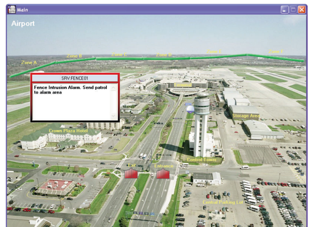
Map Window shows a visual representation of the alarm and presents the operators with instructions on how to respond to the alarm
