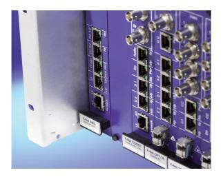
Network Management module for remote diagnostics and alarm reporting of X-Net modules via SNMP or web browser.
